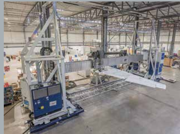
Real-scale prototype for the application of Riblets on the wing of a commercial wide-body aircraft, © 4JET.
